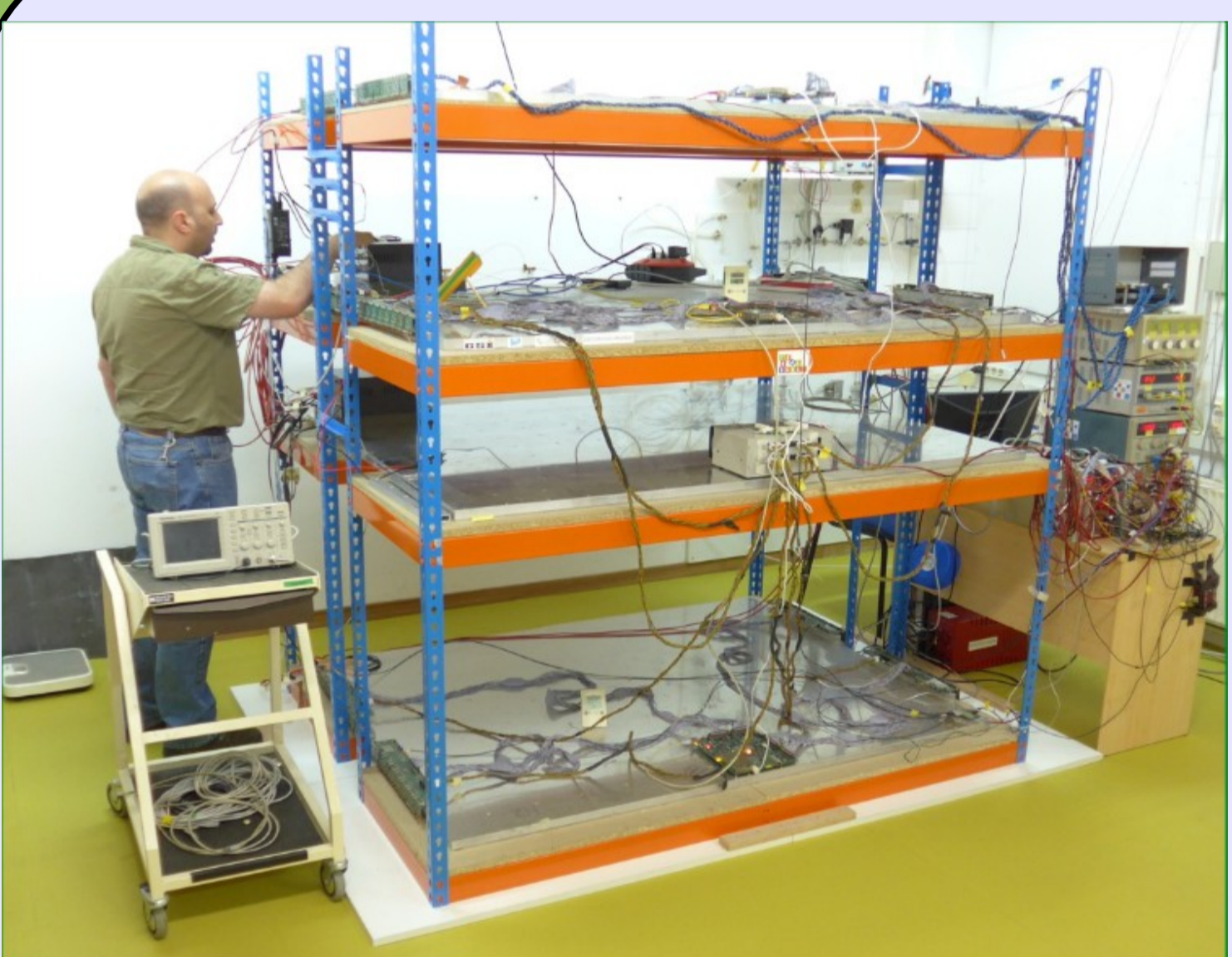
TRAGALDABAS detector at the Univ. of Santiago de Compostela. Only three of four RPC planes are instrumented. Trigger is done between planes 2nd and 4th. from the top.
