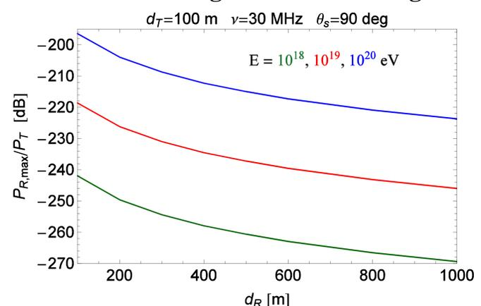
Ratio of the maximum received ( $P_{R,max}$ ) to the emitted power ( $P_T$ ) as a function of the shower core-receiver distance  $d_R$  for different shower energies  $E$ . The values of the power ratio  $P_{R,max}/P_T$  represent the strongest signal that can be attained in the MHz frequency range for  $d_T$  and  $d_R$  larger than 100 m.
