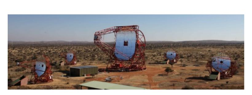
H.E.S.S. The High Energy Stereoscopic System is a Imagering Atmospheric Cherenkov Telescopes (IACT) investigating  $\gamma$ -rays from a few 10 GeV to >10 TeV.
