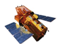
**Swift-XRT** The *Swift* X-ray Telescope is a NASA telescope firstly designed to observe GRB from 0.3 to 10 keV.
