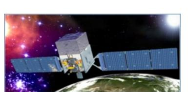
Fermi-LAT The Fermi Large Area Telescope is a pair conversion telescope designed to detect γ-rays from ~20 MeV to more than 300 GeV.
