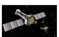
XMM-Newton The X-ray Multi-Mirror Mission is an ESA telescope to monitor X-ray sources from 0.3 to 10 keV.
