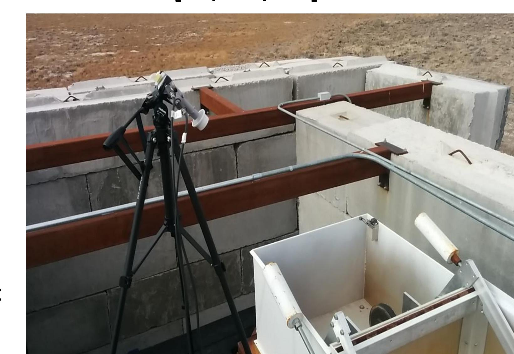
We also measured microwave intensity near the electron beam. The feed horn was fixed on the roof of the ELS without the parabola. On the ELS, various electric noises are detected depending on the status of the ELS. The largest noise comes from high voltage discharge in the Thyratron. Also noise from RF pulse in the Klystron can be seen.
