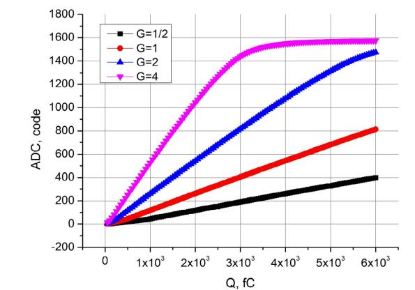
Calibration characteristics of a spectrometric tract of the ASIC MAROC3 for different preamplifier transmission coefficients.
