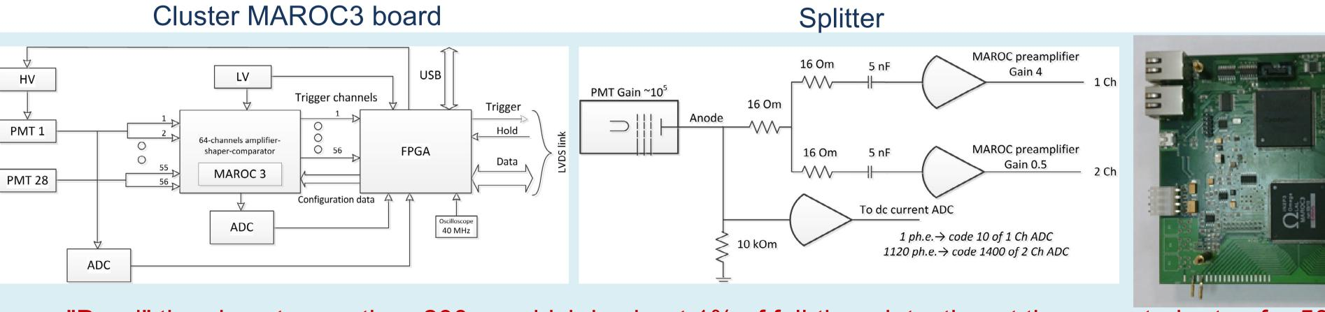
"Dead" time is not more than 200  $\mu$ s which is about 1% of full-time detection at the expected rate of  $\sim 50~\text{s}^{-1}$
