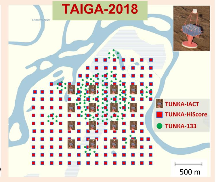
The **key advantages** of the gamma-observatory TAIGA is the joint operation of wide-angle and narrow-angle detectors of Tunka-HiSCORE and Tunka-IACT. By operating the telescopes in mono-scopic mode with distances of the order of 600 m between the telescopes, the total area covered per telescope is larger than the area that could be covered using the same number of telescopes as a stereoscopic system (requiring distances of roughly 300 m in the 10–100 TeV energy regime).
