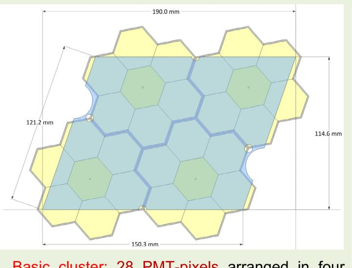
Basic cluster: 28 PMT-pixels arranged in four hexagonal cells 7HEX. The shaded area: the cross-board plate. Signal processing: PMT DAQ board based on the MAROC3 ASIC.
