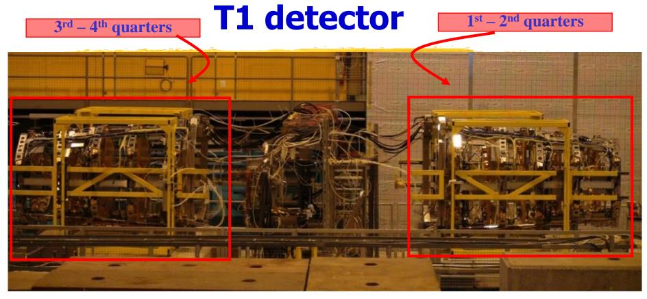
T1 telescope uses cathode strip chambers (CSC)
