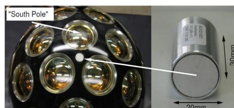
**Fig. 3** - Piezo-electric digital acoustic receiver integrated in a KM3NeT DOM.
