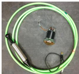
**Fig. 2** – The “external” digital hydrophone used for the LBL calibration, compared with a KM3NeT 3” PMT.
