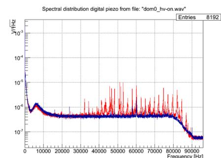
**Fig. 4** - Power spectral density of the electronic noise for an internal digital acoustic receiver as measured within a DOM in the laboratory. The blue curve shows the distribution for PMTs power off, the red curve for PMTs power on.
