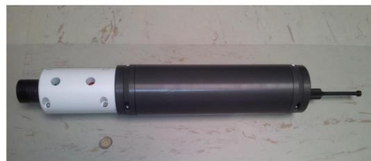
**Fig. 1** - Acoustic beacon assembly used for the KM3NeT LBL, produced by the Mediterráneo Señales Marítimas [4].
