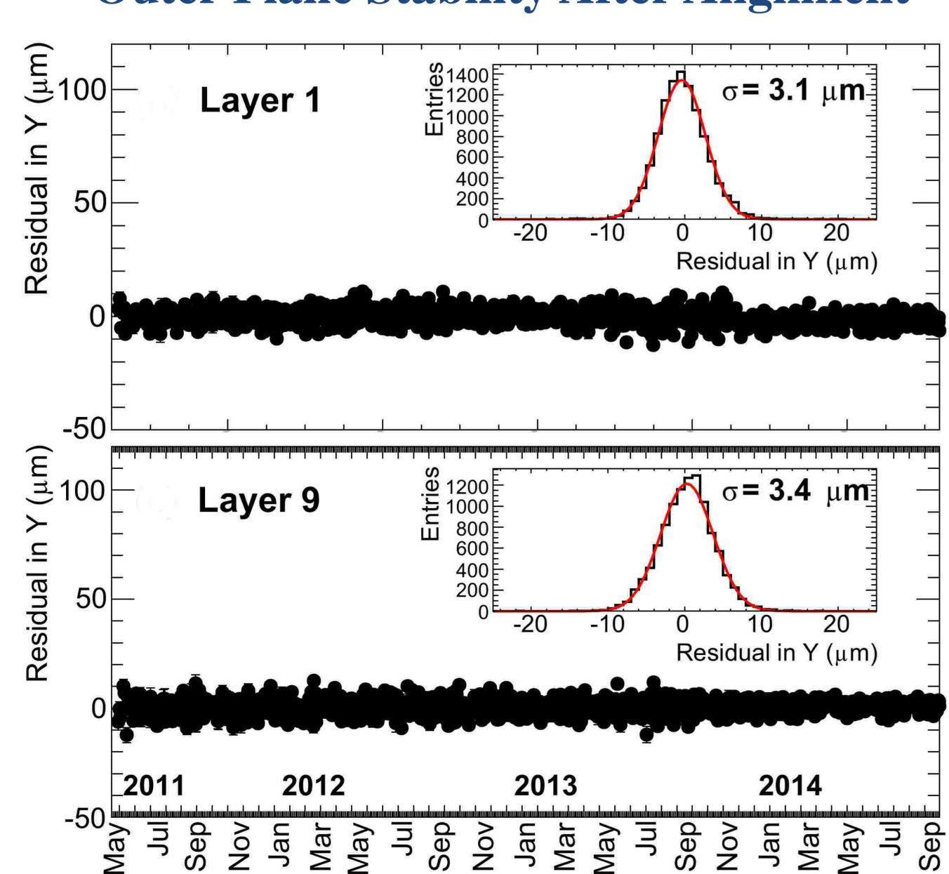
To correct for the temperature dependence, the Outer Tracker is continuously aligned with cosmic rays. Track fit residuals on the bending side are stable to 3  $\mu$ m level, well below the spatial resolution of the sensors.
