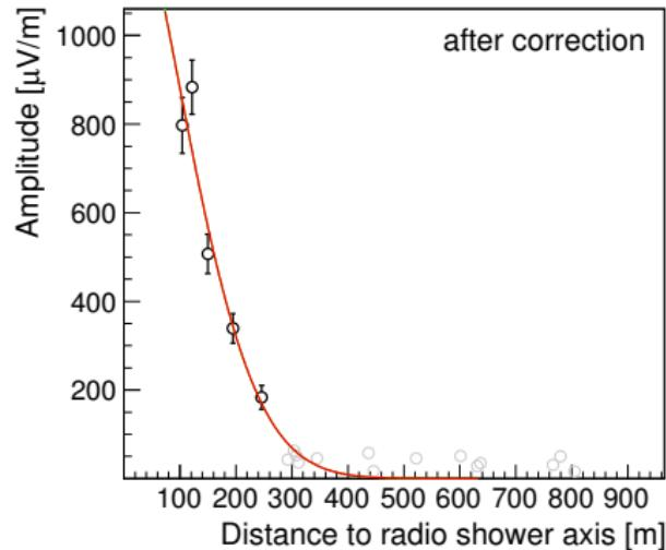
Slope ( $\eta$ ) sensitivity to shower maximum  $\delta\eta \Leftrightarrow \delta X_{\max} \lesssim 70 \text{ g/cm}^2$
