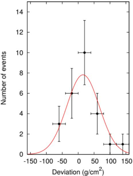
Combined resolution:  $\sigma \approx 50 \text{ g/cm}^2$  for 25 measured events
