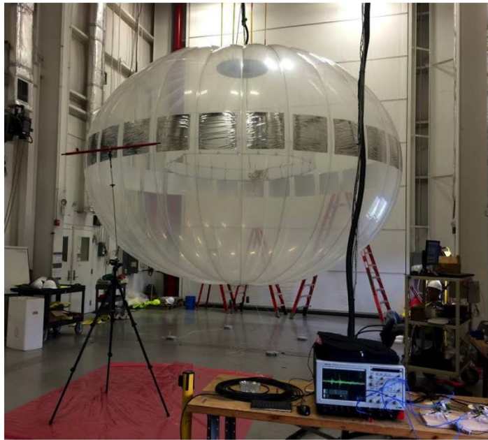
1/20 th scale model balloon. This balloon has 28 gores compared to the 280 gores of the full scale balloon.
