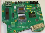
Fig. 3 — The electronic boards inside the DOM. A) Diagram and pictures of the PMT Base. B) Large and small Octopus Boards. C) The Power Board. D) The Central Logic Board.
