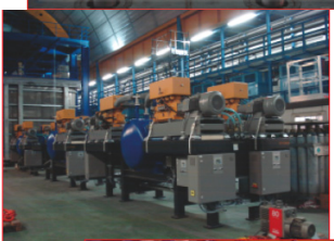
Top insulation external welding
