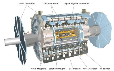
http://atlasexperiment.org/index.html S. Bentvelsen et al, JINST 3 (2008) S08003 Inner detector (±3.51 m length) Pixel detector 5, 9, 12 cm radii barrels SemiConductor Tracker (SCT) 30, 37, 44, 52 cm radii barrels Transition Radiation Tracker (TRT) 56 to 107 cm radii Calorimeter 4m radius and 8.4 m length Muon detector Outer surface of detector
