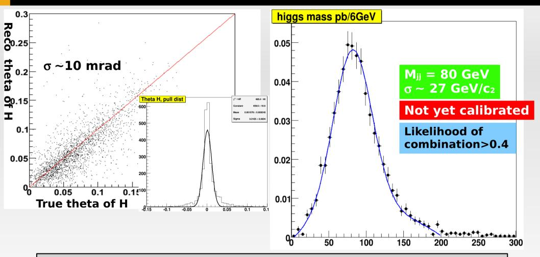
Energy of Jets\_need to be calibrated. One can initially study it with MC and then use  $Z \rightarrow bb$  events
