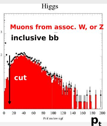
**Level 0 trigger** 88% efficient to select HW e HZ events
