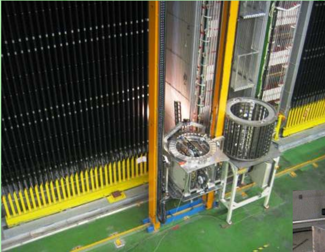
Automatic brick manipulation machine
