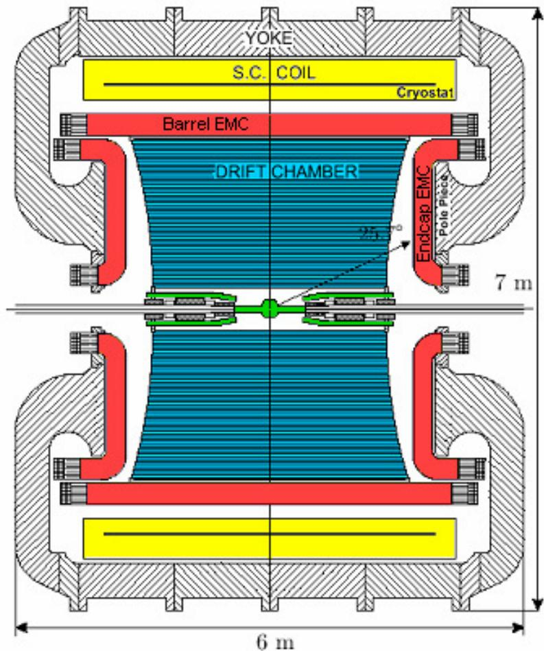
Be beam pipe (0.5 mm thick),
