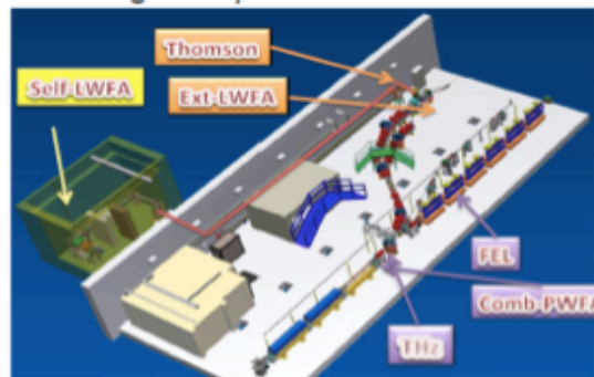
Layout of SPARC_LAB beam lines
