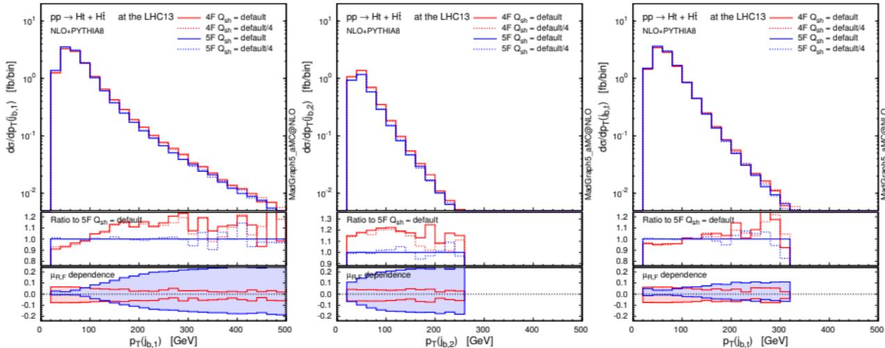
$$\text{anti-}k_T \quad p_T > 30 \text{ GeV} \quad R = 0.4 \quad |\eta| < 2.5 \quad \text{no } H \text{ decay, } t \rightarrow b\ell^+\nu_\ell$$
