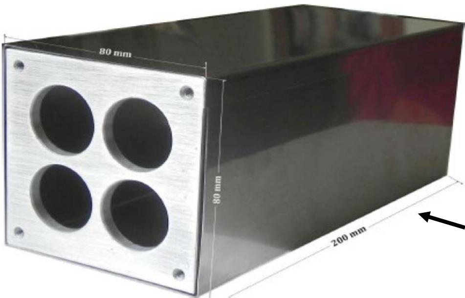
2x2 matrix of four cylindrical 0.5 inch diameter 0.5 inch long  $\text{LaBr}_3(5\%\text{Ce})$  crystals
