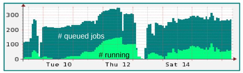
Almost no submitted jobs are declaring the expected runtime (and CPU normalization doesn't work as expected) ⇒ no efficient backfilling
