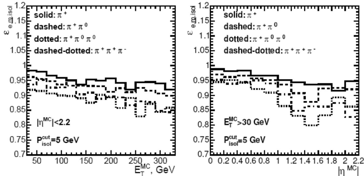
Figure 12.6: The efficiency of the ECAL isolation for  $\tau$  jets as a function of  $E_T^{\text{MC}}$  (left plot) and  $|\eta^{\text{MC}}|$  (right plot) for  $P_{\text{isol}}^{\text{cut}} = 5 \text{ GeV}/c$ . The efficiency is shown separately for different final states of hadronic decays of  $\tau$  lepton.
