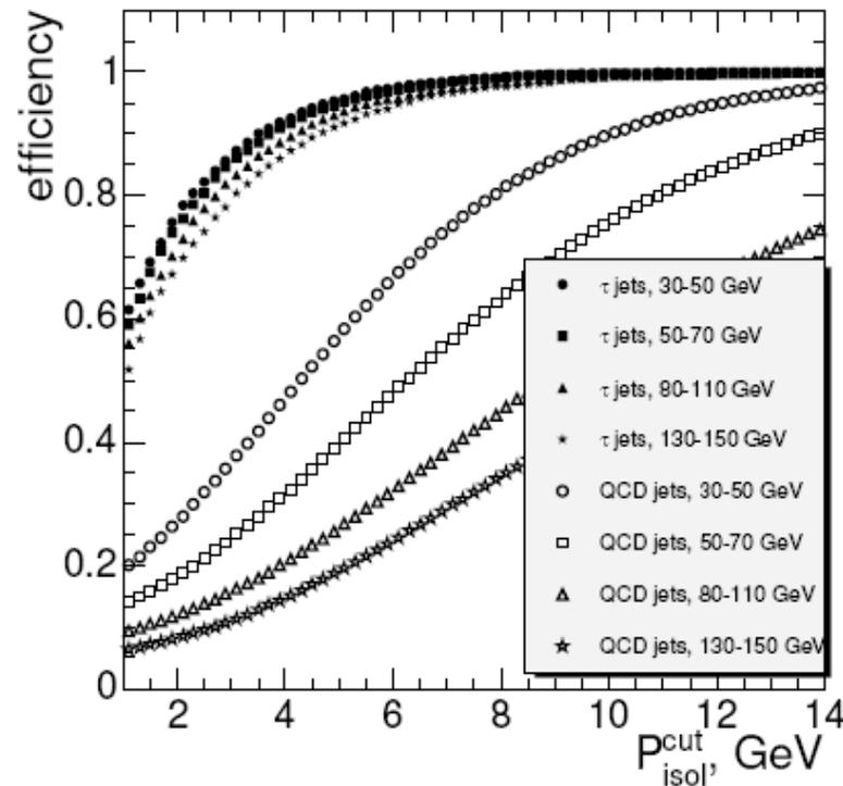
Figure 12.7: The efficiency of the electromagnetic isolation criterion, for  $\tau$  jets and QCD jets in the different bins of the true transverse energy when the value of  $P_{isol}^{cut}$  is varied.
