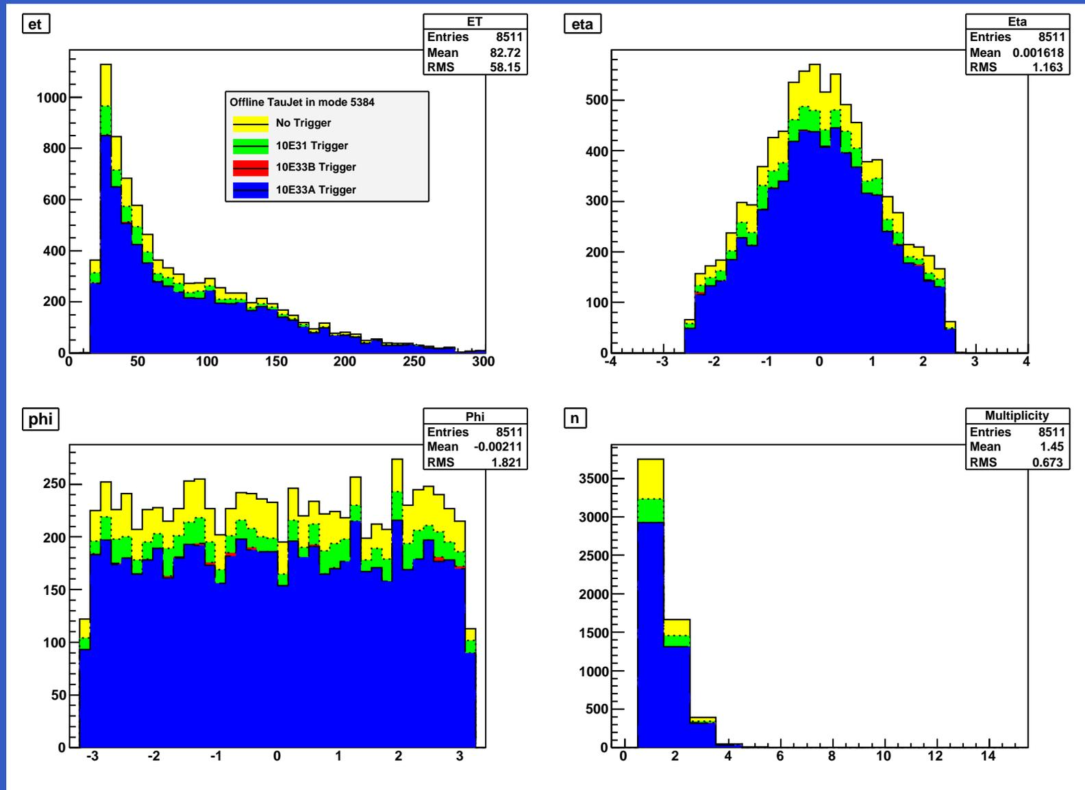
Heavy  $H_{400}^+$  with final state  $2bW_{had}\tau_{had}\nu$  offline tau distributions before and after applying the  $10^{31}$ ,  $10^{33}A$  and  $10^{33}B$  trigger. Plotted are  $\eta$ ,  $\phi$ ,  $E_T$  and multiplicity. No bias, other than threshold effects, is evident after applying the trigger menu.
