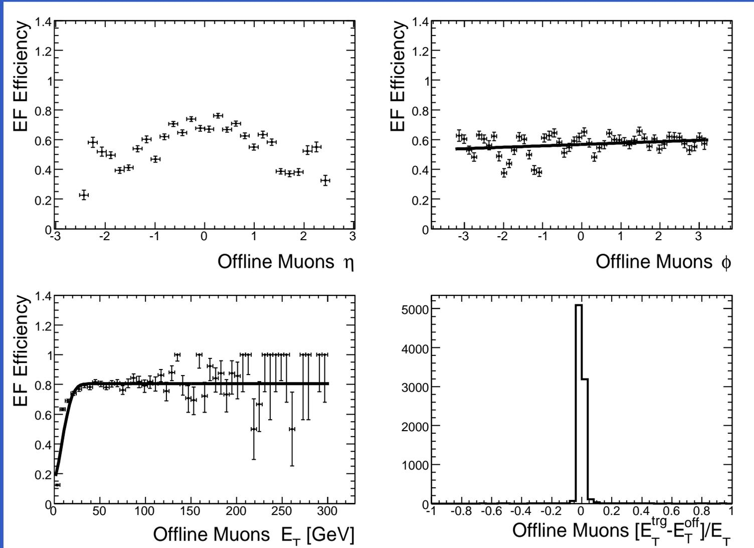
Heavy  $H_{250}^+$  with final state  $4bW_{lep}W_{had}$  trigger  $\mu$  efficiencies with respect to the corresponding offline object versus  $\eta$ ,  $\phi$ , and  $E_T$ . Resolution is also plotted. Note that the  $\phi$  efficiency for muons drops slightly on either side of  $\phi = -\pi/2$  due to the muon spectrometer feet.
