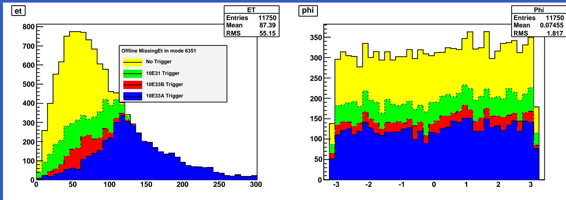
Light  $H^+$  with final state  $2bW_{had}\tau_{lep}\nu$  offline  $E_T^{miss}$  distributions before and after applying the  $10^{31}$ ,  $10^{33} A$  and  $10^{33} B$  trigger. Plotted are  $E_T$  and  $\phi$ . No bias, other than threshold effects, is evident after applying the trigger menu.
