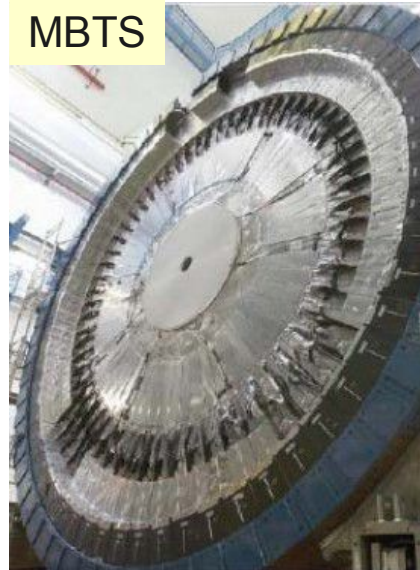
Minbias Trigger Scintillators mounted on LAr cryostat 32 sectors (individual or multiplicity triggers) Main trigger for initial running period
