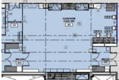
Class 1,000 Clean Room GEM Assembly Lab
