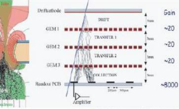
GEM foils developed using PCB manufacturing techniques
