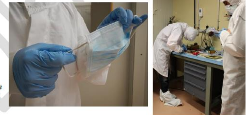
Fig 17: example of clean room mask (left) and dressing (right)
