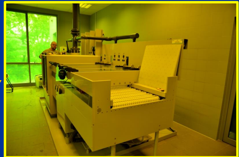
New Cu etcher (350l main chamber)
