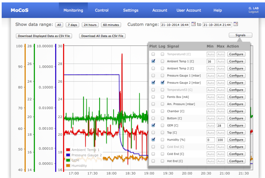
Figure 7: Trend graph configuration: Clicking on the "Signals" button above the graph opens the configuration popover. There you can select which channels should be plotted and if they should be plotted logarithmically and specify minimum and maximum y-values for each axis.
