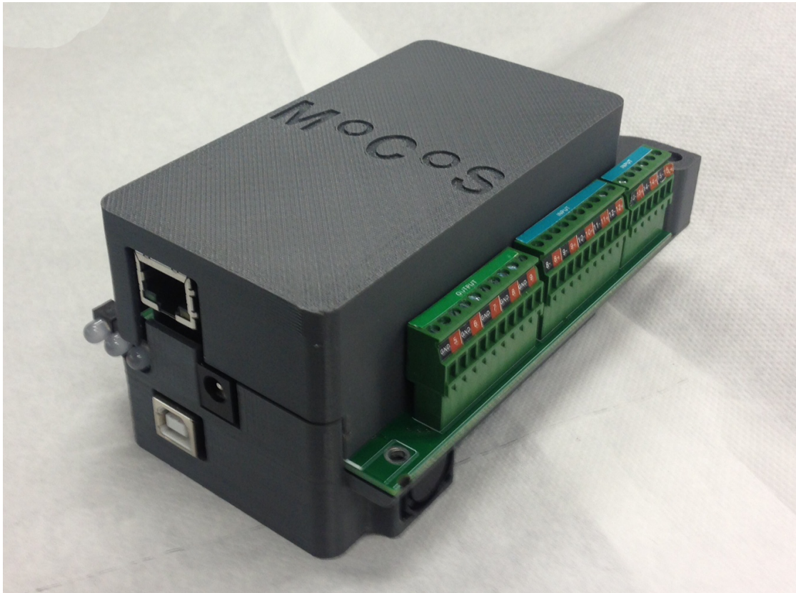
Figure 2: Standalone device: The portable, standalone version of the MoCoS device is housed in a 3D printed case and has its connectors arranged all around the device.
