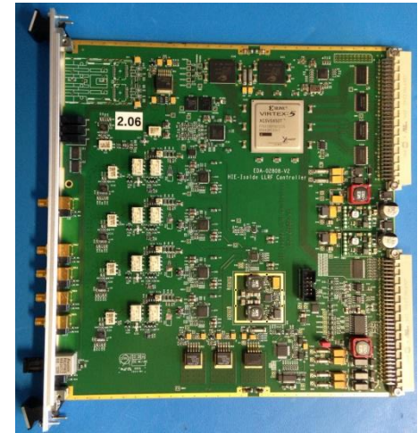
LLRF system for a complete cryomodule (6 cavities)
