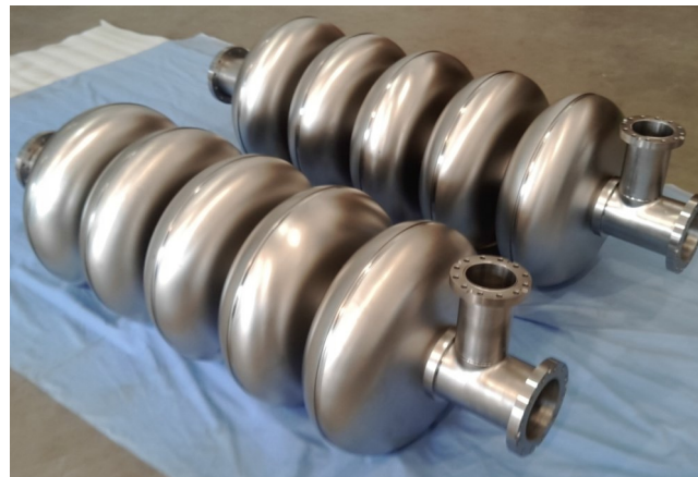
650 MHz \beta=0.82 5-cell cavity vertical test soon
