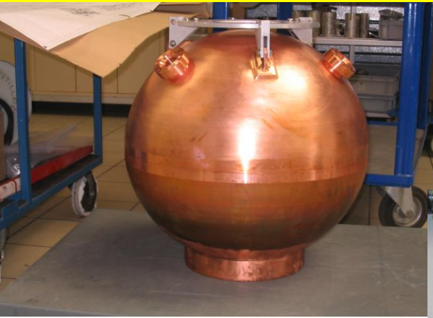
Low background detector d=60 cm p=10 bar
