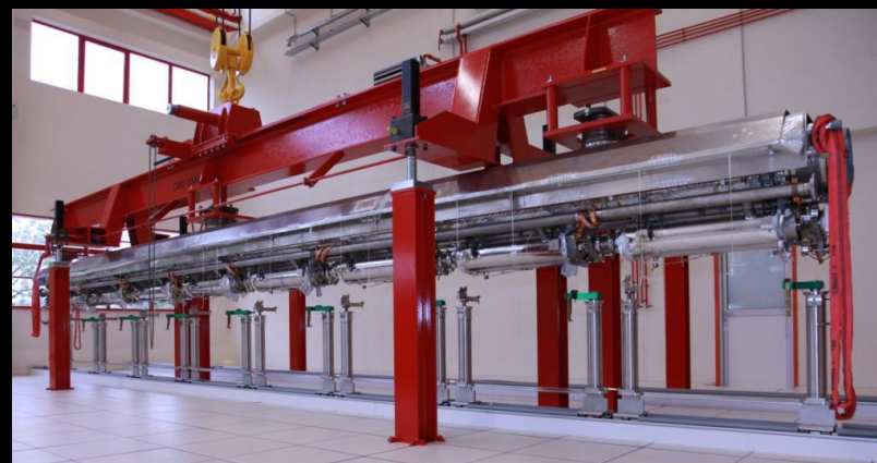
Transfer of cryomodule in clean room roll-out area
