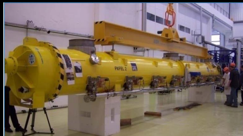
Transfer of cryomodule in RF coupler assembly area
