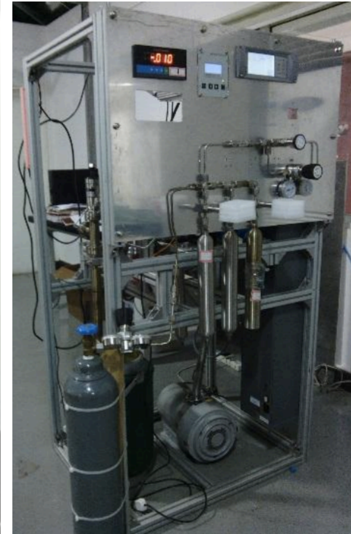
a cold-trap system to measure Kr/Xe down to ppt level
