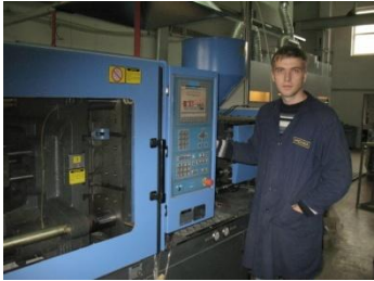
Injection-molding of scintillation plates
