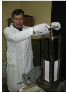
Assembling of ECAL modules
