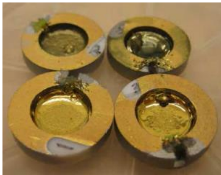
Detector 7 mm \phi x 5mm deep
