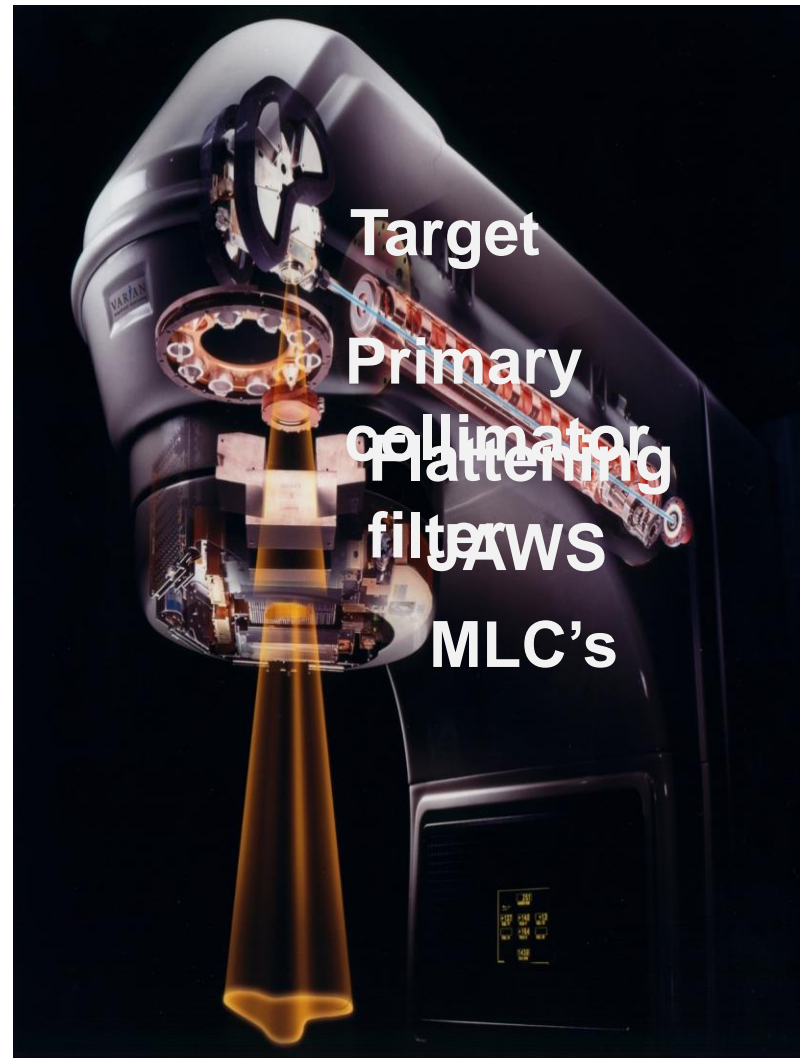
Figure 1: Varian 18MV Medical Linac cross section view. [3]
