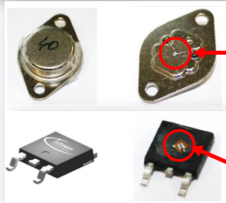
SPD04P10P prior and after etching
