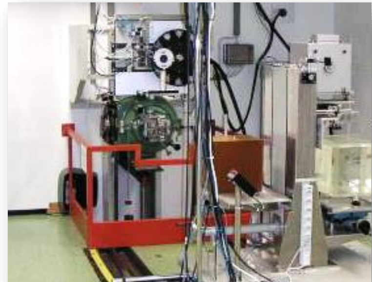
Co-60 TID Radiation Exposure Facility EN/ISO IEC 17045 Test Lab, Seibersdorf
