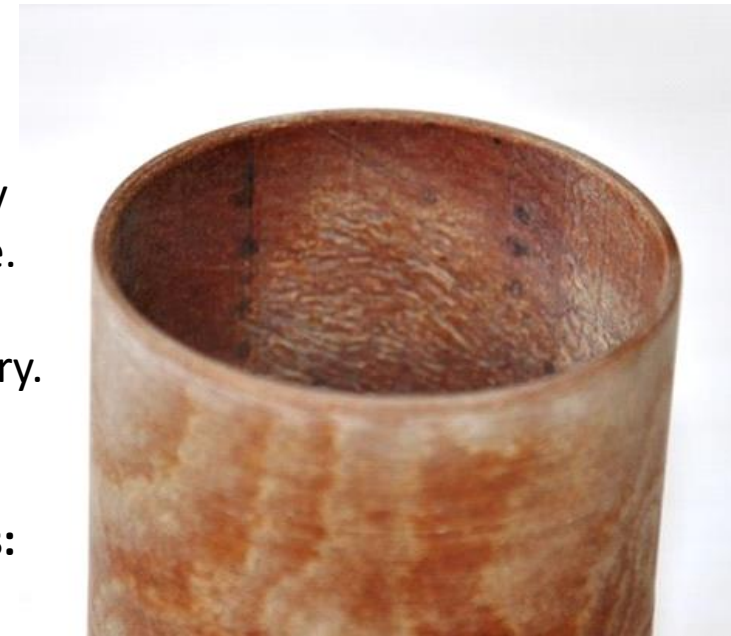
Sand blasted Bakelite tube after sparking
