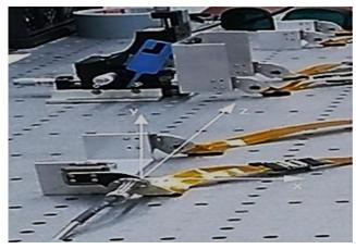
The preliminary results: the displacement measurement of the tested elements  $\,$  was measured with precision at the level of  $\,20~\mu m$
