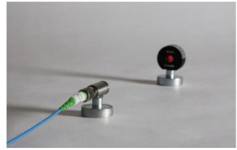
ETALON - the current characteristics: range 0.2 -20 m, multiple simultaneous 3D measurements with uncertainty of 0.5μm/m
