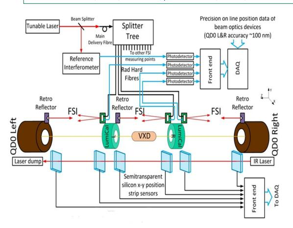
FSI - the absolute distance measurements between two parts of LumiCal detector.
