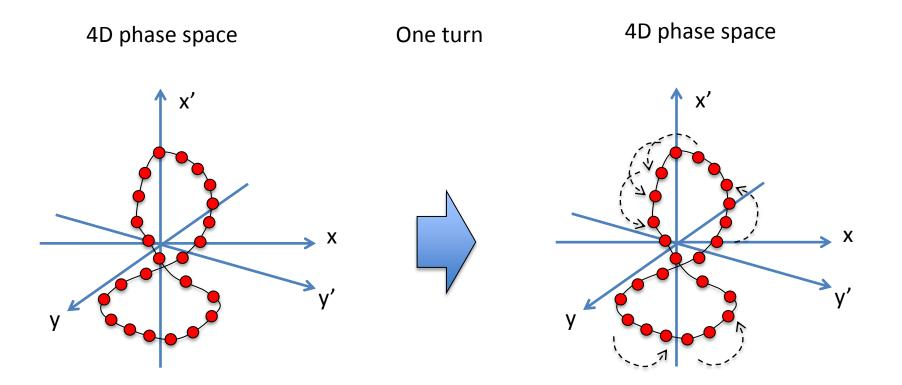
After one turn each point on the fix-line is mapped into the fix-line
