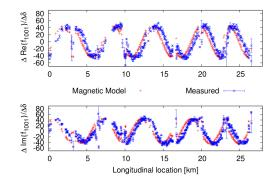
Small phase shift: perhaps due to enhancement of errors in IRs at lower β\*
