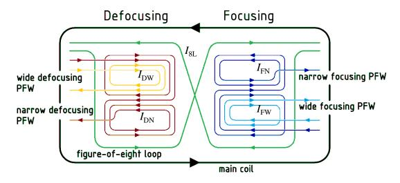
PS magnets model used for tracking reproduces PS Main Units by a combination of multipole kicks.
