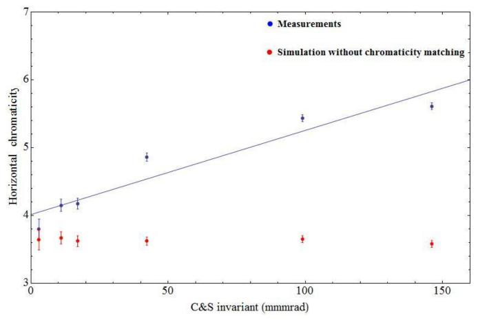
PS model does not reproduce the linear chromaticity increase with kick amplitude.
