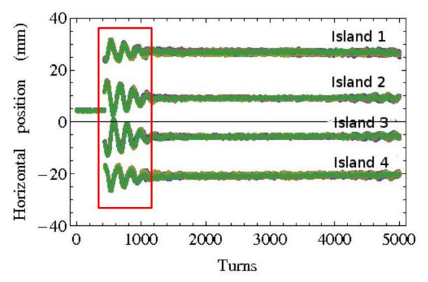
The filamentation just after kick into islands allows us to probe the island optics conditions.
