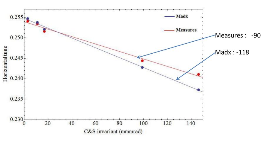
A second discrepancy appears after calculation of linear chromaticity vs kick amplitude extract from decoherence analysis.
