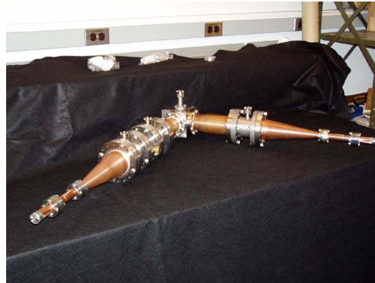
Ka-band component assembly, including barrier window, miter bend, pump-out sections, tapers, and mode converters. Transmission efficiency of the assembly is 95%.
