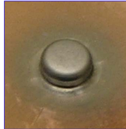
Tungsten Insert After RF Processing to 419 MV/m (Pulse Length: 150ns)
