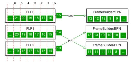
**Approach**: Delay first sending of some FLPs by an offset, storing pending messages in a buffer.
