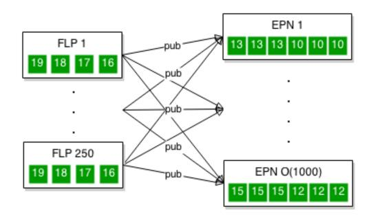
All FLPs sending at the same time to a single EPN could overload the network path.
