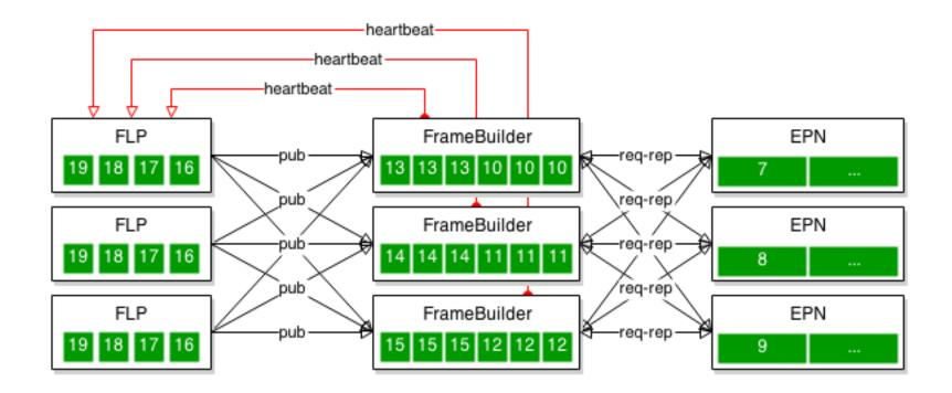
FrameBuilder: separate device to collect timeframes together.
