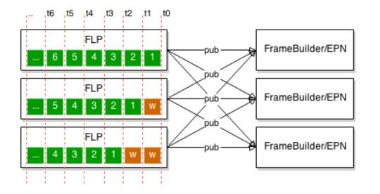
When the buffers are full, all FLPs can send at the same time; payloads go to different EPNs/Frame Builders.
