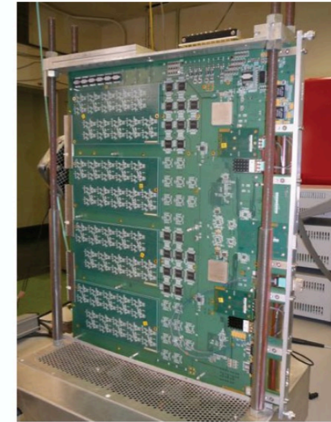
Digital motherboard, analog mezzanines
