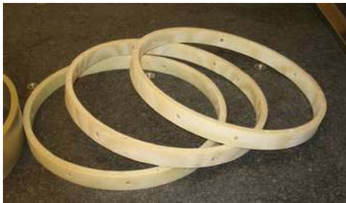
Permaglass annular flanges outside the active area act as supports for the detector
