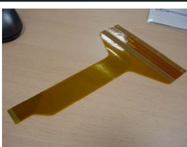
25 \mu m kapton with resistive layer for cryogenic application
