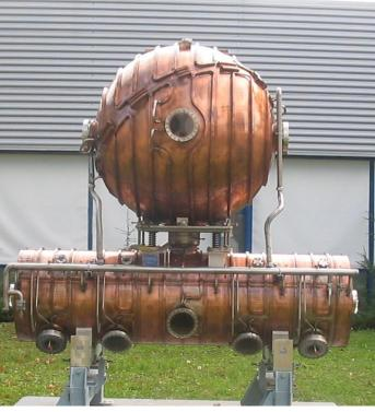
**Essential**: resonant cavities (with storage cavity on top) provide necessary acceleating field (compensate synchrotron losses)
