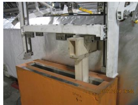
Lifting of BRAN (model) with HXTC Crane And BRAN fixture.
